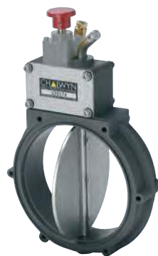
STOP BUTTON (VALVE MOUNTED OPTION) AIR PRESSURE CONNECTION RESET LEVER TO LATCH OPEN
